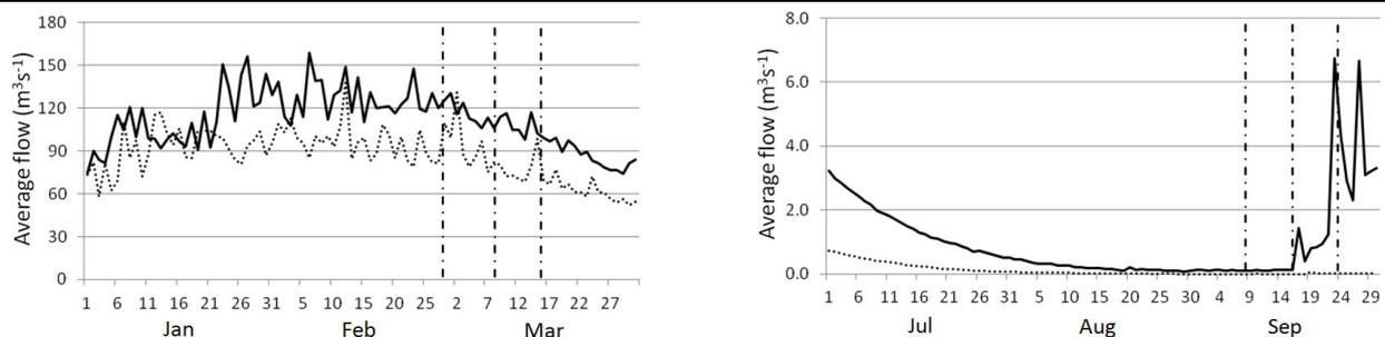
Figure 2. Estimated average daily mean flow for wet (left plot) and dry (right plot) seasons in Vouga River (solid line: flow in reference conditions; dotted line: flow in projected conditions; 1<sup>st</sup> dashed-dotted vertical line: equinoctial tide; 2<sup>nd</sup>: neap tide; 3<sup>rd</sup>: spring tide).
