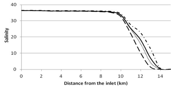
Figure 4. Maximum salinity along Espinheiro channel at equinoctial tide (black dashed line: A0 scenario; black solid line: A1 scenario; black dotted line: A2 scenario; black dashed-dotted line: A3 scenario).
